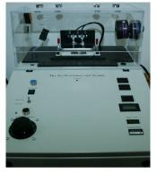
6-Series: The LEC 6-Series test system provides simplified performance of Dust-and-Fog Tracking and Erosion Resistance of Electrical Insulating Materials in accordance with ASTM D2131 (D 2131). The three test sample system allows for unattended operation after initial setup and configuration of the test samples.
